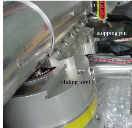
Fig. 4 – Sliding joint for easy assembly.
