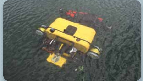
HAUV can be operated in remote mode via a tether
