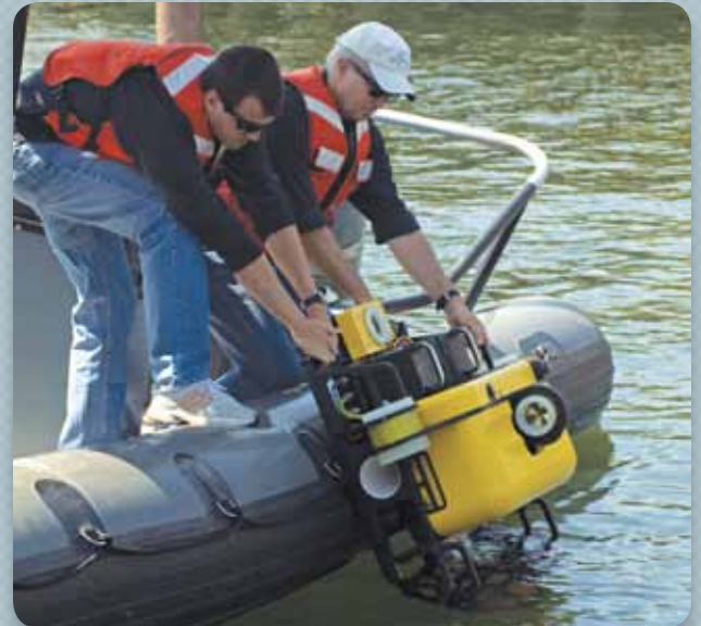
HAUV can be easily launched and recovered from a small boat
